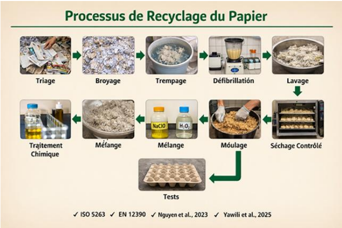
Figure 2: Process Flow for Cellulosic Waste Transformation and Tray Fabrication
