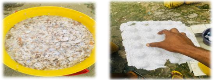
Figure 3: Defibrillation and Molding Stages (a) Intermediate pulp suspension showing partially disintegrated fibrous bundles; (b) Formed molded fiber egg tray specimen after mechanical dewatering.
